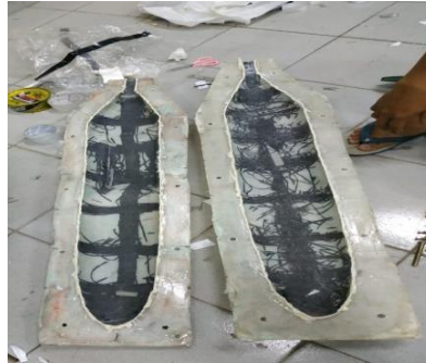
Gambar 1. Hasil cetak fuselage fiberglass
