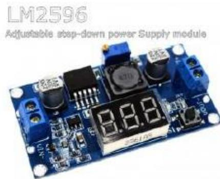
Gambar 5. Modul Step Down
