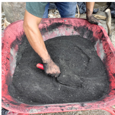
Gambar 6. Proses pencampuran paving block geopolimer
