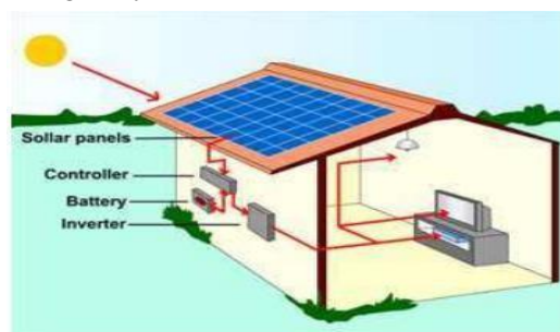
Gambar 1 Instalasi Panel surya
