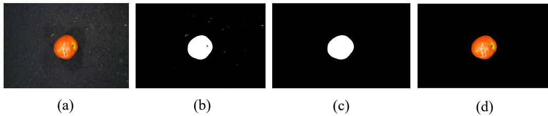
Figure 4: Result Image after (a) RGB Conversion, (b) Segmentation, (c) Morphology and (d) RGB Clean Segmentation
