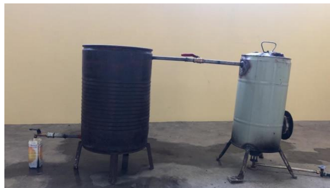
Gambar 2. Proses pirolisis biochar cangkang kelapa sawit
