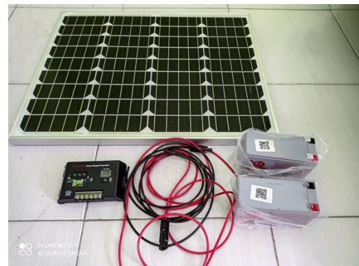
Gambar 3. Panel Surya, Charge Controller dan Battery
